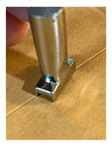
By placing the impressions like this it gives you the right angle for the basket weave to run and still have the overall pattern flow parallel to the reference line. So in this case since center line runs parallel to the edges of the money clip, the design will run parallel to the borders and all the stamp impressions should be even with the borders when we are finished.
