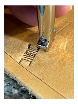
Just like I showed in my Straight Basket Weave tutorial, we want to leave a slight gap between the back of the stamp and the center bar of the last impression. The arrow in the picture below shows this gap. It's just a small gap, only about the width of the thickness of the leg impression. This allows us a little leeway to keep things straight and keep the stamps from crowding as we go.
